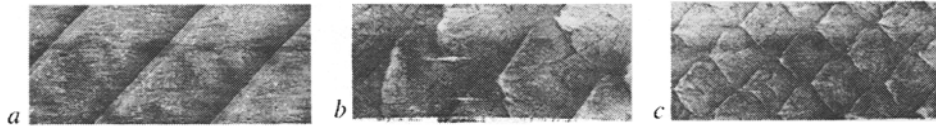
Fig. 4. Trace impressions of states of the detonation-wave-front structure for detonation modes with the following orders: a) N = 0 , P_0 = 53.2 mm Hg; b) 1 and 139.8; c) 2 and 158.1 (a C_2H_2 -air stoichiometric mixture).
